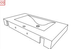
KKR can help clients open the bracket and screw holes in advance.
