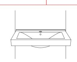
Secure the sink to the wall with the mounting brackets and screws. After inserting the first fastener, verify that the sink is level. When the sink is properly aligned insert the remaining fasteners.
