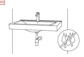
Connect all supply tubes to the faucet. Turn on the water supply to check for any leaking from the water supply lines or sink.
