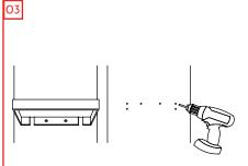
Determine the height you want. Place basin against the wall. Use a level to make sure both sides are level. Mark location and drill on wall for mounting holes.
